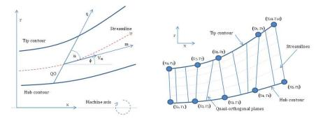
FIG. 4.1. Meridional view of the flow path (left panel), and Steam path design geometry (right panel).
